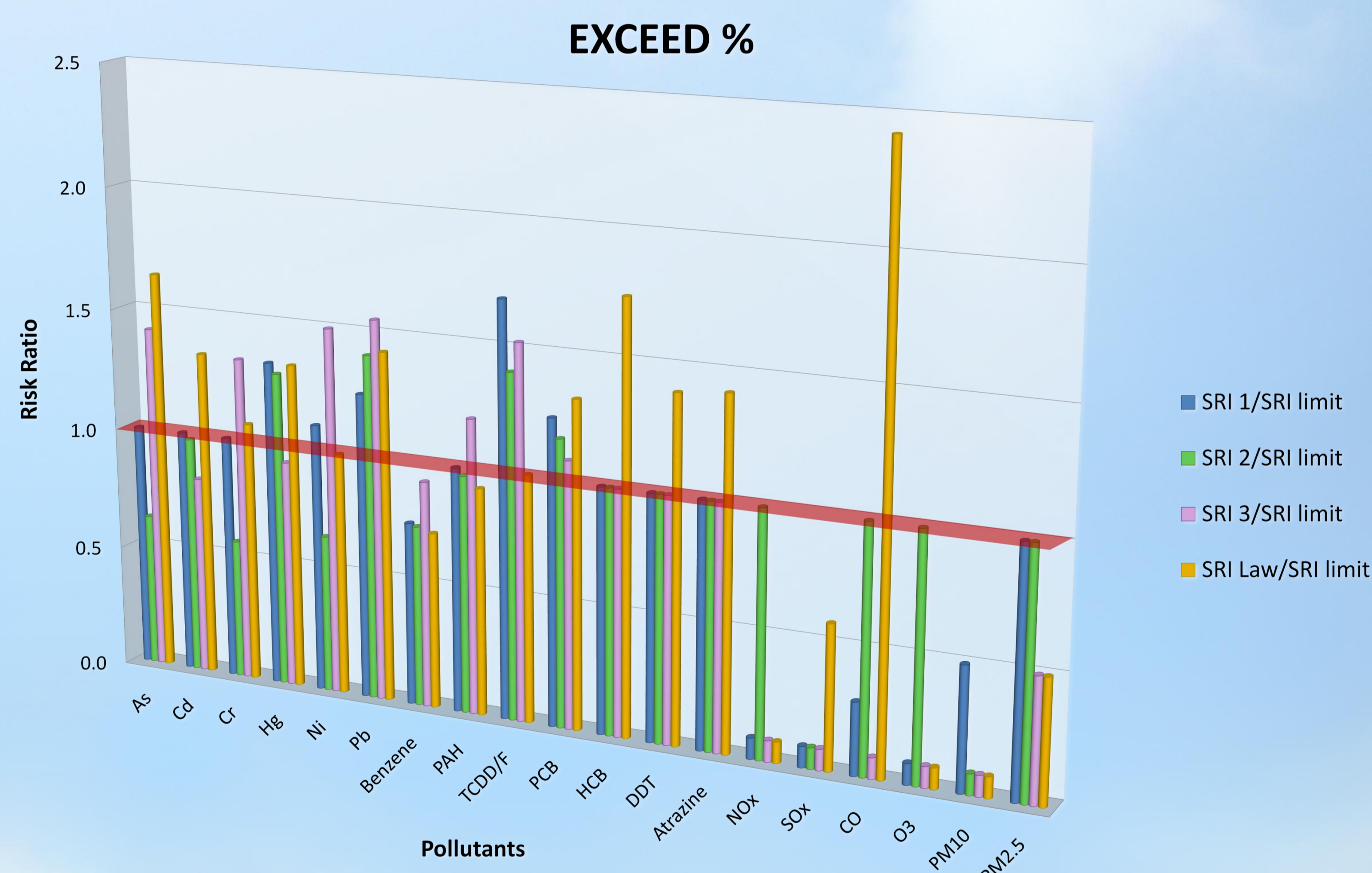
Fig. 2 : Risk distribution of 19 pollutants used in the 3 case studies and legal limit case. Red line shows the risk threshold for environmental status
